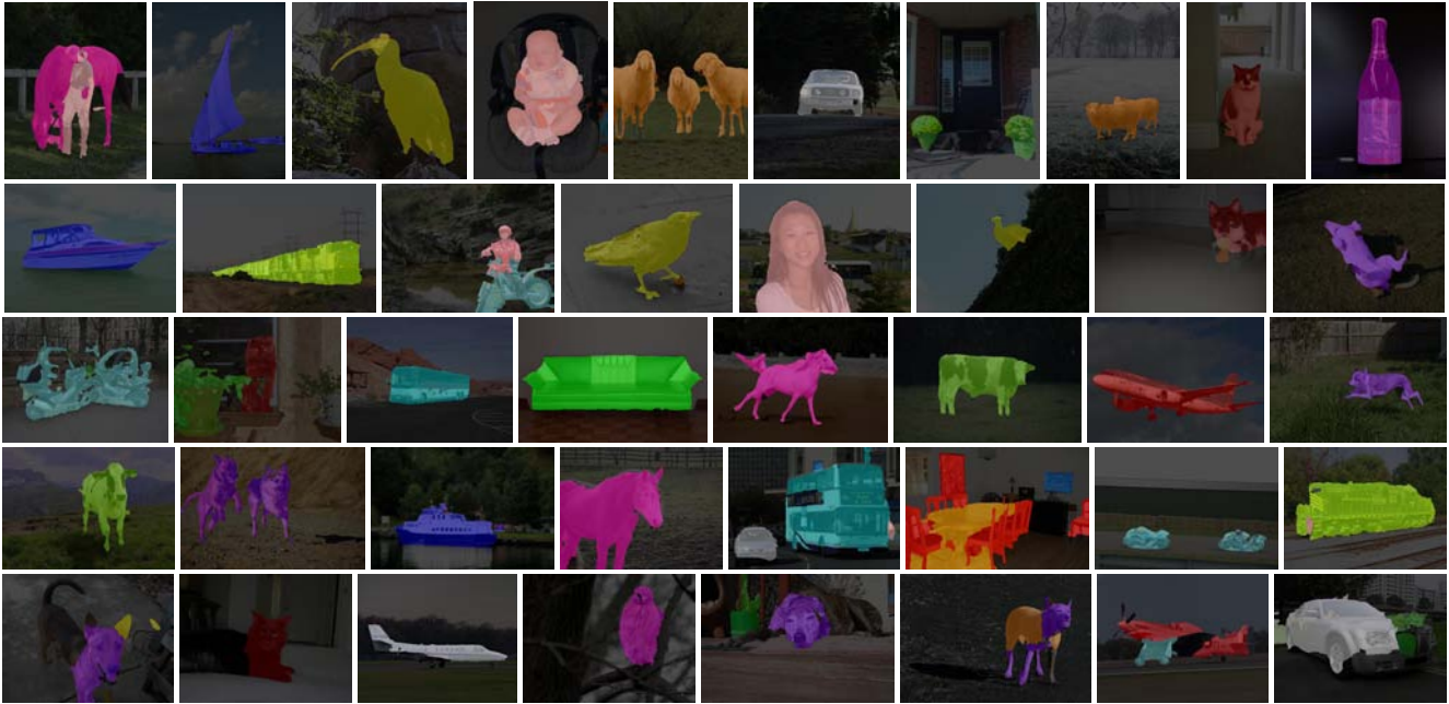
Figure 9. Results on the Pascal VOC 2010 test set are usually pixel-accurate if the object is well detected. Failure cases, as shown in the last row, are mainly due to problems of the detector. Object completion requires a sufficiently homogenous object or background.
