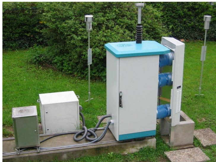
Figure 3.7: The pollenmonitor in the measurement field of the German Weather Service in Freiburg. The image was taken on April 28th, 2006.
