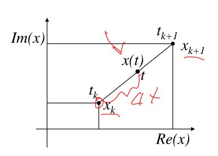
$$x(t) = \underbrace{x_k + \underbrace{(x_{k+1} - x_k)}_{\Delta x_k}} \frac{\Delta t}{t_{k+1} - t_k}$$
