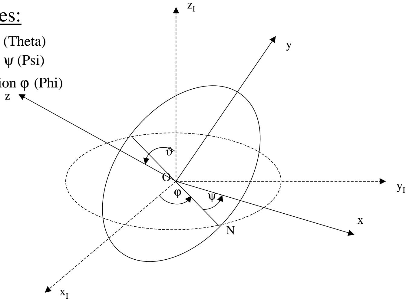
To exchange from the inertial system into the body coordinate system the following three rotations are needed:
