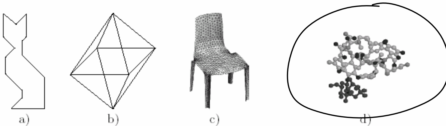
Fig. 1. Discrete structures in 2D and 3D: (a) closed contour described by a polygon (b) wireframe object (c) 3D triangulated surface mesh (d) molecule.
