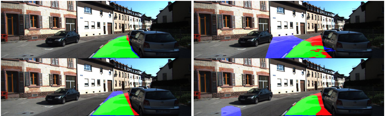
Fig. 5: Lane predictions on the KITTI dataset compared with the 3 next best approaches. Top Left: Our approach, Top Right: ANN, Bottom Left: PCA-Lane-S, Bottom Right: S. In the images green is correct segmentation, red false negative detection and blue positive detection.
