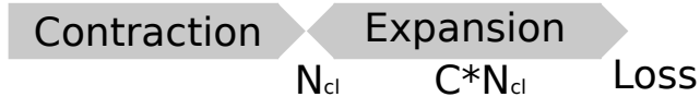
Fig. 3: Description of the new architecture weight distribution. The expansive side increases its parameter size by a factor of C . Only the convolutional layers between the contraction and expansive side and before the loss continue with N_{cl} filters.
