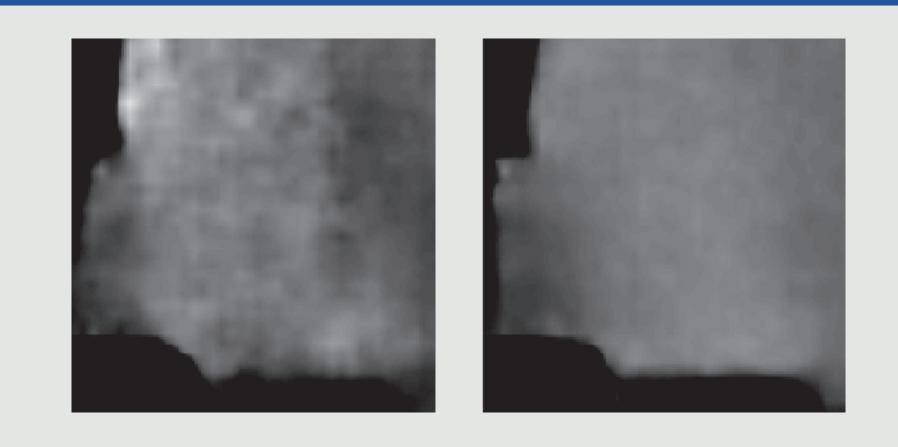
Close-up of a predicted disparity map without (left) and with (right) convolutions between up-convolutions.
