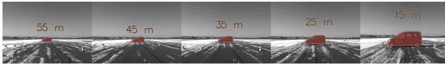
**Fig. 7. Segmentation and distance estimation from monocular video.** The segmentation and distance estimation of the stationary obstacle proves to be precise throughout the video sequence. The early detection and localization of the obstacle leaves time to induce obstacle avoidance strategies.
