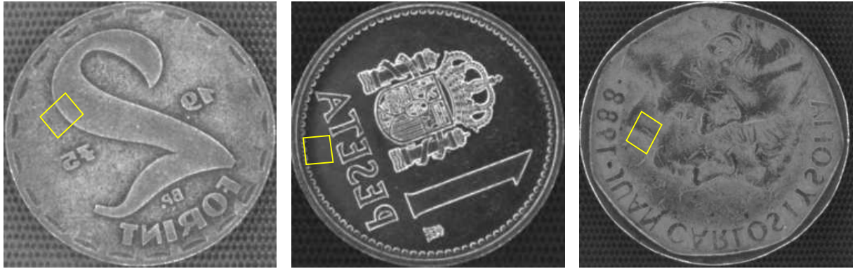
Figure 2: Abrasion effects. Due to abrasion several slight gradients are introduced near the edges. Not only the edges contain structural information that may be considered, also putatively flat regions contain valuable structure. Our algorithm also uses this information for recognition.
