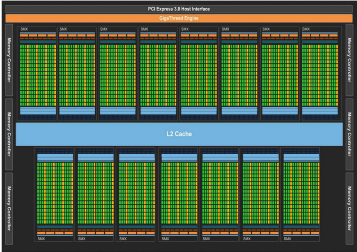
Figure 4.2: Organization of multiprocessors in a modern GPU [20]
