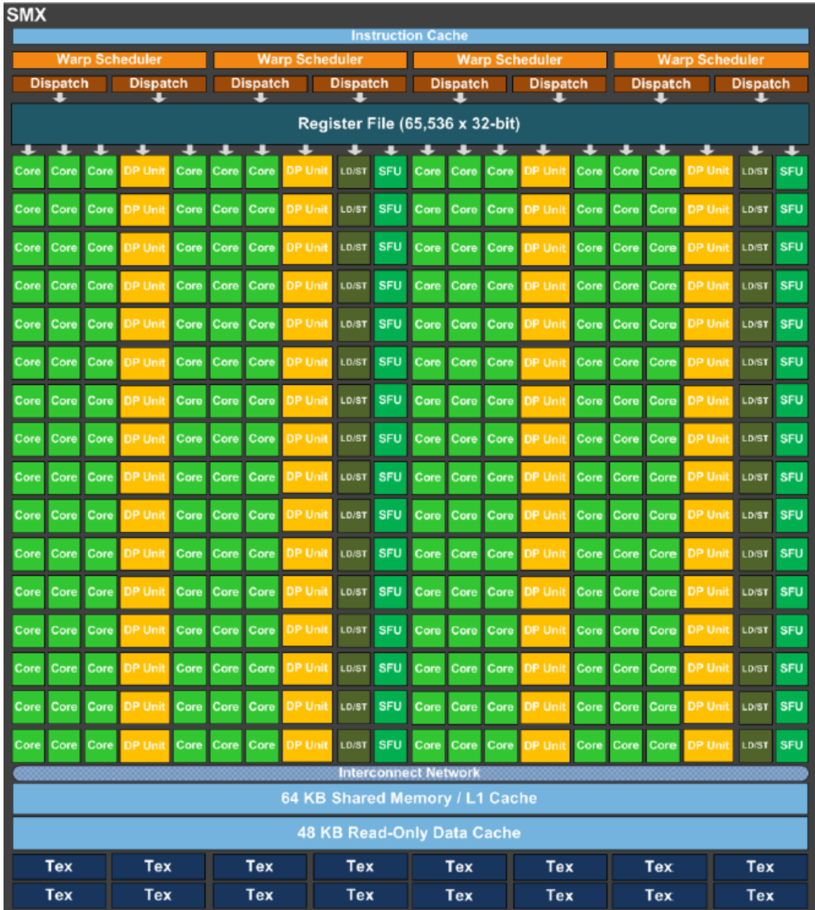
Figure 4.3: Organization of a streaming multiprocessor in a modern GPU [20]
