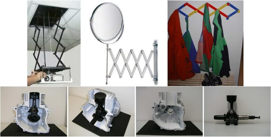
**Fig. 2. Top:** Examples for a pantograph type of constrained kinematic chains to lift projectors (left), to adjust a cosmetics mirror (middle), or a wardrobe for children (right). **Bottom:** The second example: a rotating crankshaft and piston in a one cylinder engine assembly. Both types of constrained kinematic chains will be used in the experiments.
